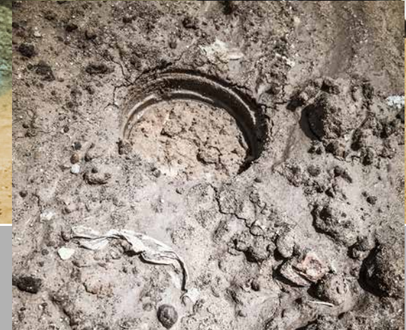
Photo above shows soil coated and penetrated with HydraGuard 21 where a core sample has been removed, noting penetration of HydraGuard into the soil
