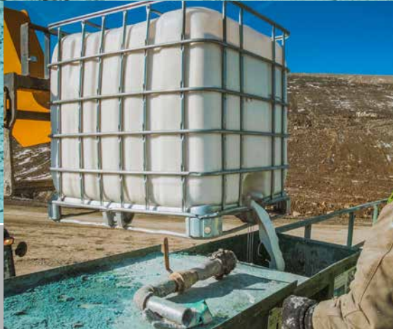
Loading HydraGuard into a Hydroseeder using a extending forklift.
