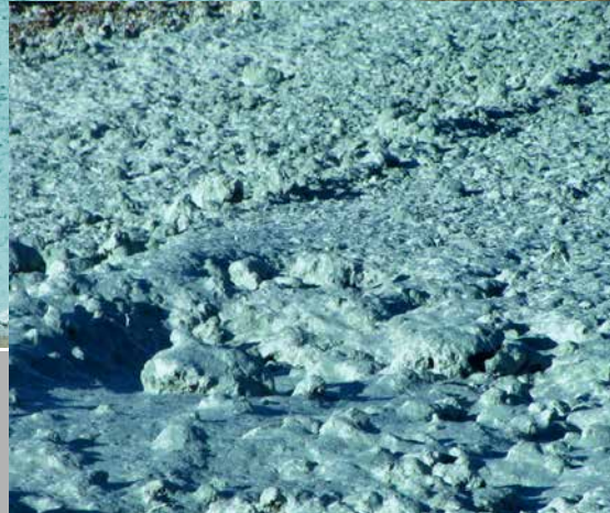
Impact of HydraGuard blended with chemistry used in ConCover SW Superplus. Note the thickness and density of the cover material
